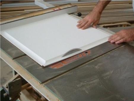
**Step 1** In order to get the desired effect, only one side of the panel should ever be cut. First you should measure the width of the finished panel. Rip the one side down to the desired width. The height will always remain the same at 24".
