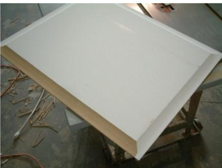
**Step 3** :: You will now sand the newly cut radius using a fine grit sand paper. This will remove the rough edges left by the router and will give you a finished surface for painting
