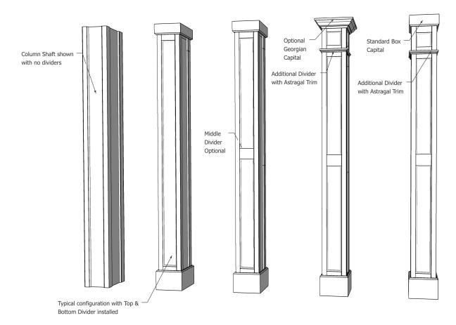
Please note we include MDF glue for Wood columns, and PVC glue for PVC columns. Dividers for fibreglass columns are made from PVC, however the PVC glue will not work when adhering PVC to Fiberglass. PL Premium or any Construction adhesive is recommended, but is not included, with the Fibreglass columns.
